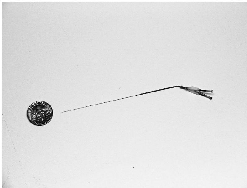
**Fig. 4.** Microdialysis needle. This 32-gauge device has the size, shape, and handling properties of an acupuncture needle and, likewise, is designed to be minimally invasive. (Shah JP, Phillips TM, Danoff JV, Gerber LH. An in vivo microanalytical technique for measuring the local biochemical milieu of human skeletal muscle. *J Appl Physiol* 2005 Nov;99(5):1977–84. Epub 2005 Jul 21. Original is Figure 2 on page 1978 of article.)
